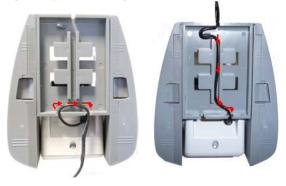
Please refer to the arrows depicted on the bottom of the base when placing the cables, detailed in Figure 3.
