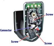
Carefully lift out the gold contacts circuit, and remove the battery holder while letting the white connector pass through the hole in the battery holder (as shown below).
